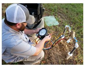
directly to the water system must install and maintain a backflow prevention device. This device prevents water from flowing backward and re-entering the main water supply. A backflow prevention brochure is available by calling 731-422-7500.
