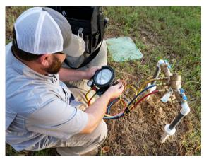
directly to the water system must install and maintain a backflow prevention device. This device prevents water from flowing backward and re-entering the main water supply. A backflow prevention brochure is available by calling 731-422-7545.
